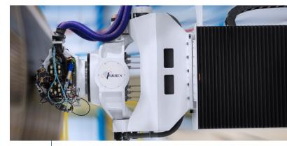
TORRESFIBERLAYUP machine manufactures high-contour carbon fiber aircraft components.
