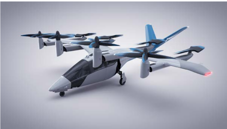
Vertical Aerospace’s VA-1X has a winged design that gives it lift and reduces electrical load when in flight.
