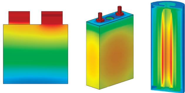
Electro-thermal model of cells of different geometries.
