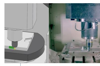
Sandvik Coromant simulates its machining processes in a virtual setting using the **3D**EXPERIENCE platform before sharing them with its customers.
