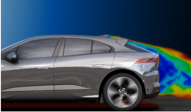
Realistic rendering in SIMULIA PowerVIZ – Jaguar I-Pace aerodynamics
