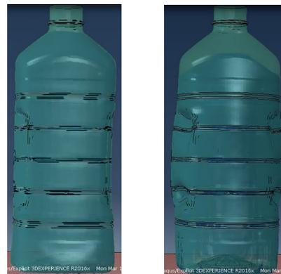
Simulation of container bulging when dropped.
