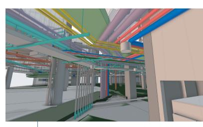
Top image: CATIA Fluid 3D Systems Designer on the **3D**EXPERIENCE platform enables designers to view 18 floors of mechanical, electrical and plumbing (MEP) elements at fabrication level of detail (LOD) 400 on what will be the world's tallest wood building.
