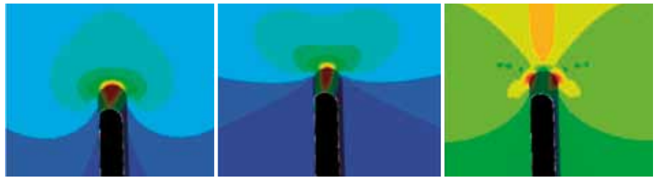
Figure 1. FEA of the stress distribution around the expansion joint of the process vessel skirt support shows equivalent stress (left), circumferential stress (center), and axial bending stress (right).
