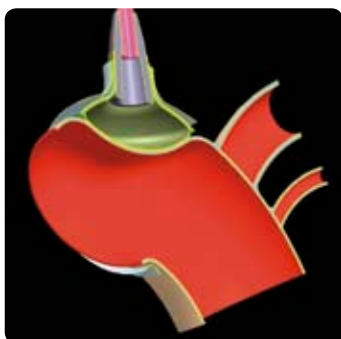
Image 3: Pro/Engineer Geometry of C-Pulse unit on which Matrix’s Abaqus FEA models were based.
