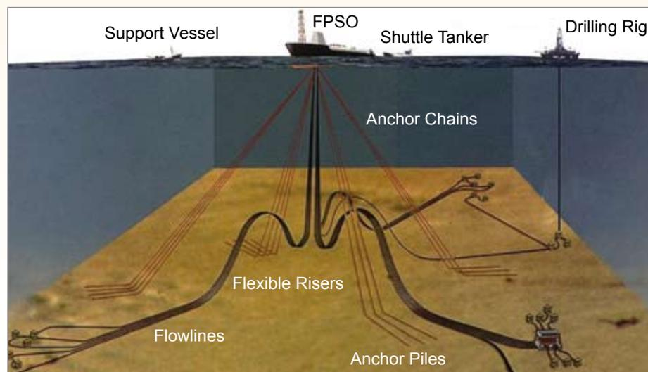
Diagram showing intended applications of DeepFlex pipe in deepwater installations. All-composite flexible fiber-reinforced pipe can be used for dynamic risers, subsea flowlines and pipelines, subsea jumpers, and surface jumpers on hybrid risers or on platform decks.
