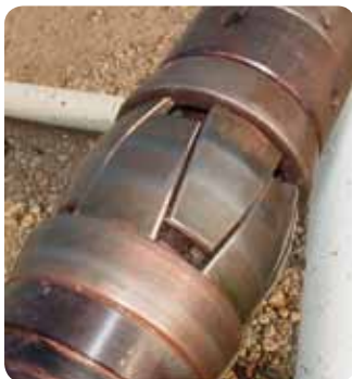
Segmented expansion cone.
