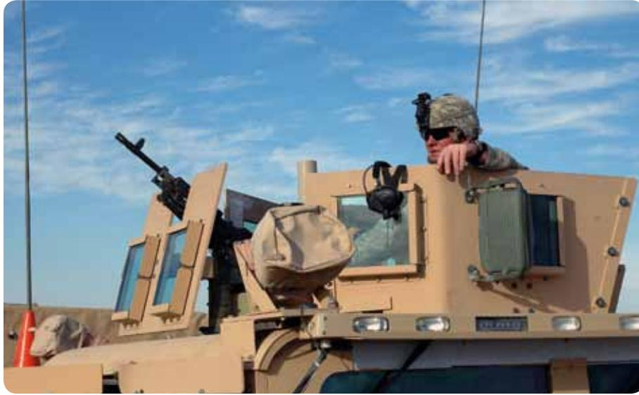
The Objective Gunner Protection Kit mounted atop a combat vehicle.
