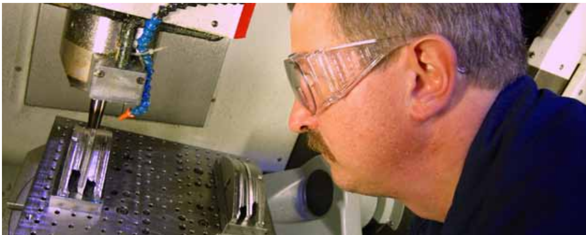
CATIA model data drives the 5-axis mill used for high-speed machining of the optical insert finish.
