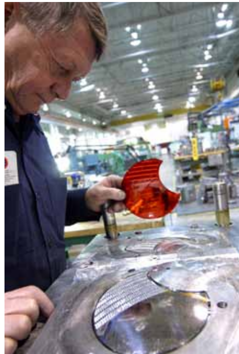
Incorporating publications into designs with CATIA CAA Extended Development allows departments throughout DBM Reflex to use that knowledge. Here, an assembly technician checks the fit of a two-section lens on the mold used to produce it.
