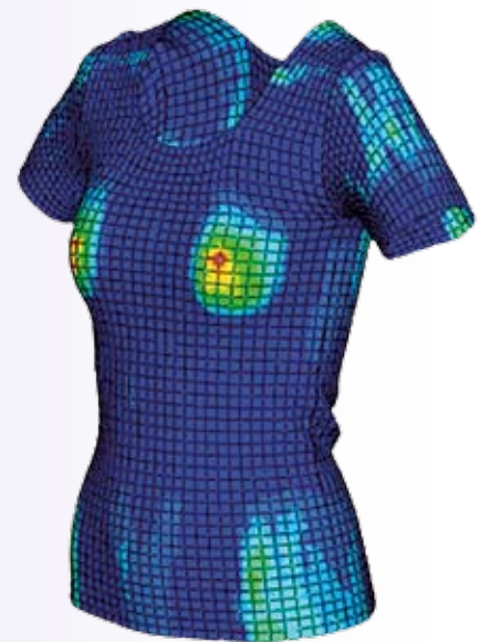
Figure 3. Clothing pressure distribution from Abaqus simulation results for a t-shirt.
