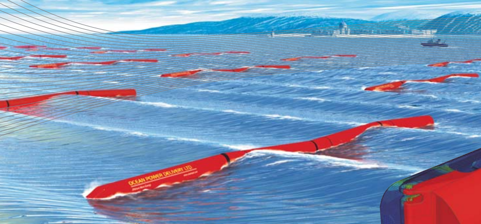
The Pelamis is a semi-submerged floating structure, composed of cylindrical steel sections linked by hinged joints.
