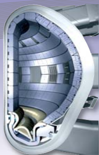
Cross-section of vessel and internal components
