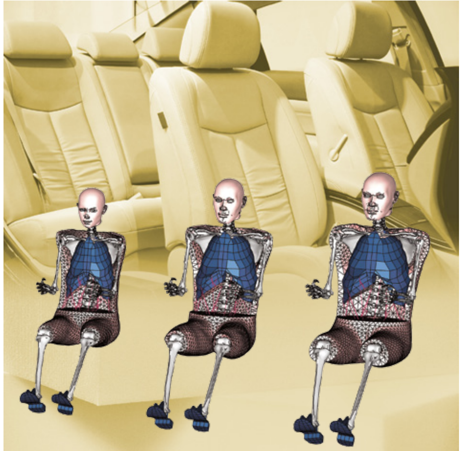
Figure 1. The CASIMIR family of human-body models includes several versions determined by the height and weight percentile that they represent: f05 corresponds to a small female; m50 a man in the 50th percentile; and m95 a large man. Adaptations can be made to account for physical variations of other nationalities and races, and an individualization algorithm further customizes the model.
