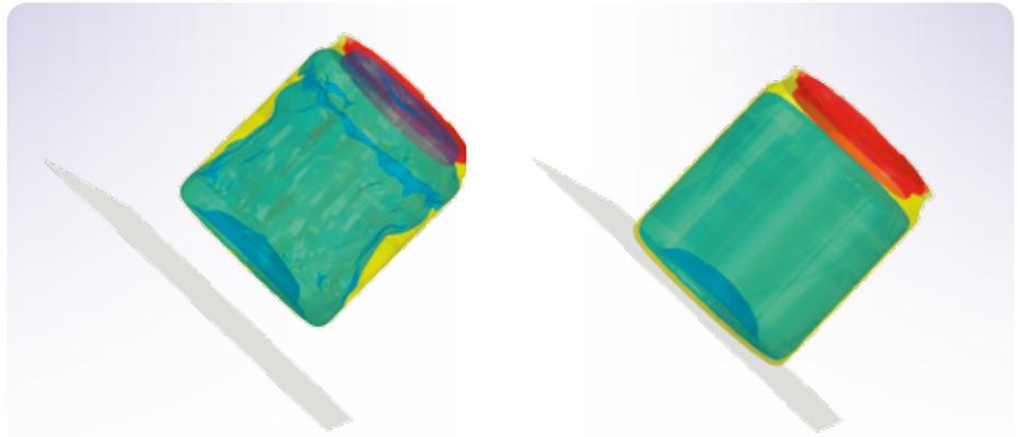
Abaqus FEA container drop test uses a coupled Eulerian-Lagrangian analysis to show the interaction between the container, the fluid it holds, and the surface it impacts. The top must stay on even when the container is dropped 3 ½ feet to a hard floor.
