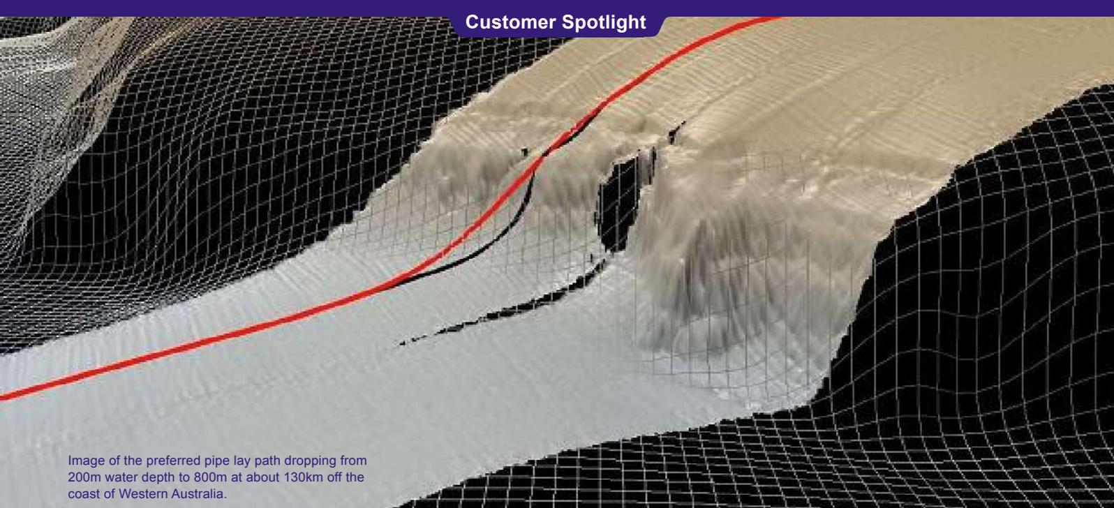
Image of the preferred pipe lay path dropping from 200m water depth to 800m at about 130km off the coast of Western Australia.
