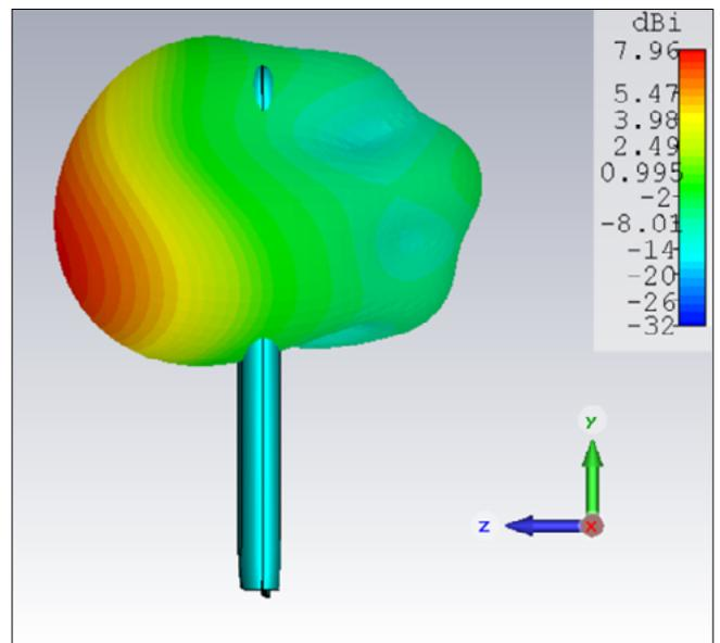
Figure 3: Radiation pattern of the Freevolt antenna inside the CleanSpace tag.
