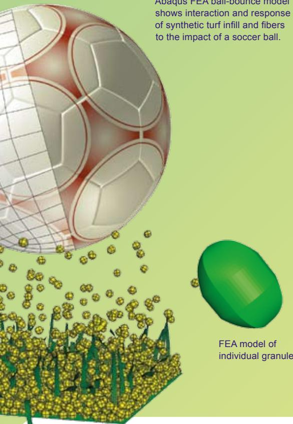
Abaqus FEA ball-bounce model shows interaction and response of synthetic turf infill and fibers to the impact of a soccer ball.
