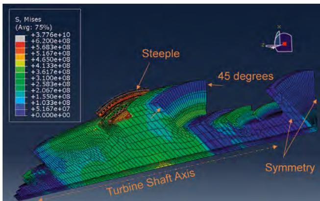
Turbine shaft, one-eighth symmetry 45 degree model with cracks examined at several locations.
