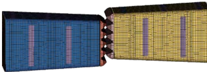
Side view of two aluminum crash modules modeled in Abaqus FEA software to simulate a crash. The impact is offset to determine whether the teeth at the front of the modules can prevent either module from climbing over the other. Vertical stripes on the module sides represent trigger slots, points of weakness built in to induce controlled plastic failure.
