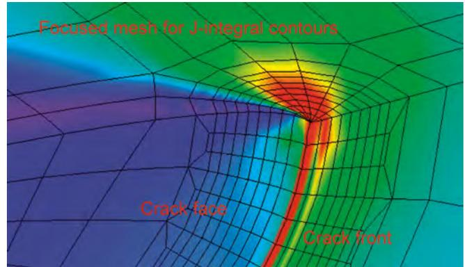
Close-up of the focused mesh along the crack front for Abaqus to compute J-integral results in each contour.
