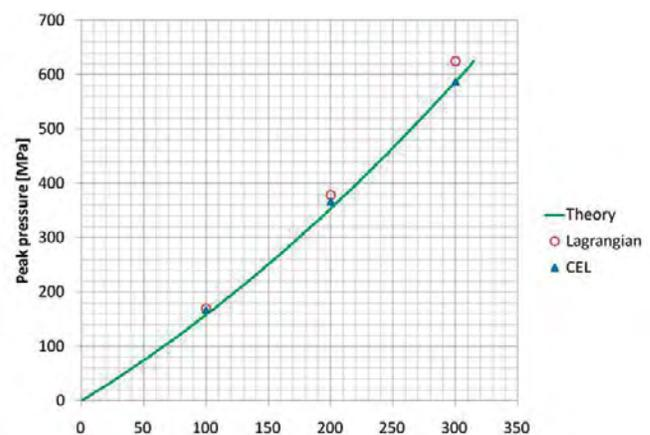
Comparison between the theoretical, CEL, and Lagrangian peaks of pressure for the cylinder
