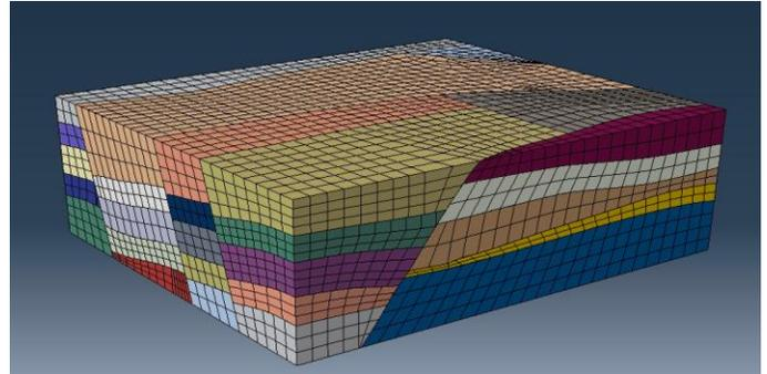
Figure 4: A model containing horizons and faults created using the second workflow. Both, Abaqus/CAE as well as CATIA, are used for creating this model.
