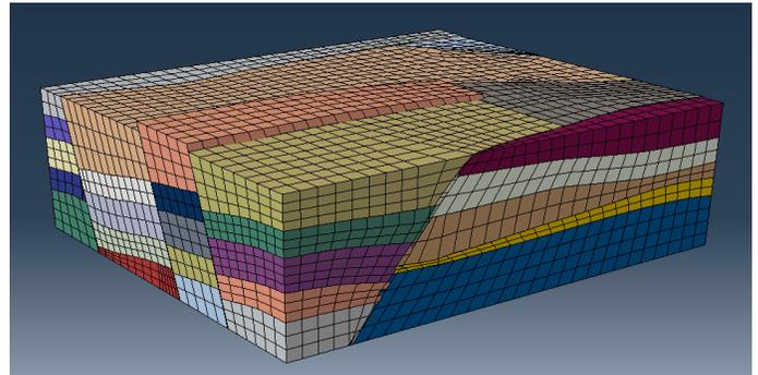
Figure 11: Fault slippage due to changes in pore pressure near a geological fault. Compare with Figure 4, which shows the undeformed configuration.
