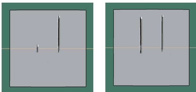
Figure 10: Hydraulic fractures in the formation after the propagation of the right fracture, shown on the left, and then the propagation of the left fracture, shown on the right. The analysis has been done using the extended finite element method (XFEM) and using a coupled pore fluid flow displacement formulation. The fractures are seen to extend vertically upwards due to the reduction in the lateral stress at higher elevations.
