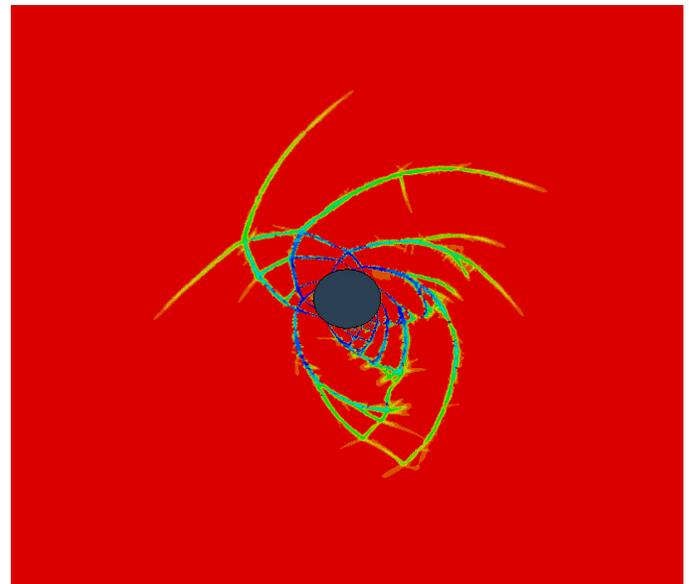
*Figure 7: Shear band pattern computed using the newly implemented orthotropic clay plasticity model. The analysis is for a bore-hole model subjected to in-ground stress and insufficient mud pressure to support the rock. The rock fails in shear as the mud pressure is reduced.*
