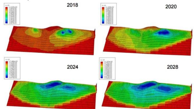
Figure 5: Four increments in an Abaqus FEA simulation of subsidence in a hypothetical oilfield, displayed over ten years (Ref. 2). Blue areas denote greatest downward displacement of
