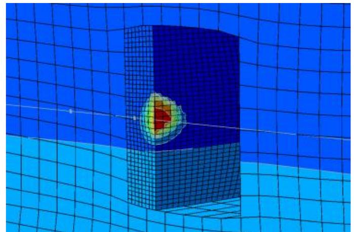
*Figure 8: Pore pressure contours in a hydraulic fracture stimulation analysis based on the new pore pressure cohesive elements that exhibit smooth transition between Darcy flow and Poiseuille flow. Gravity effects are included in this element formulation.*
