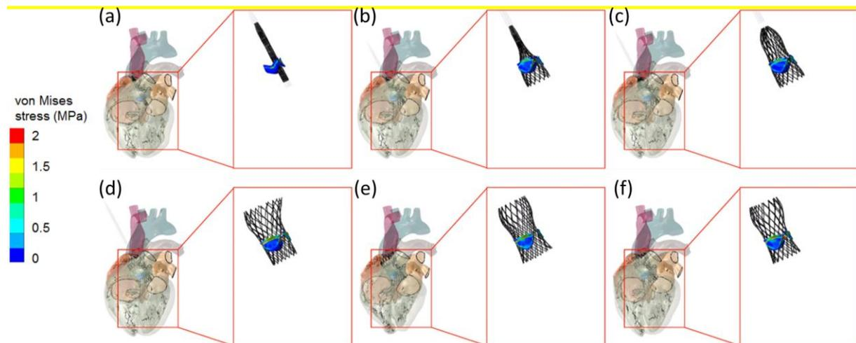
**Fig. 3 Medtronic *CoreValve* stent expansion in the LHHM with calcified aortic valve: (a) pushing of the leaflets to open position with the stent and the crimper, (b, c) self-expansion of the ventricular and aortic parts of the stent, respectively, (d) fully deployed stent, (e) beating phase, and (f) recovery phase.**
