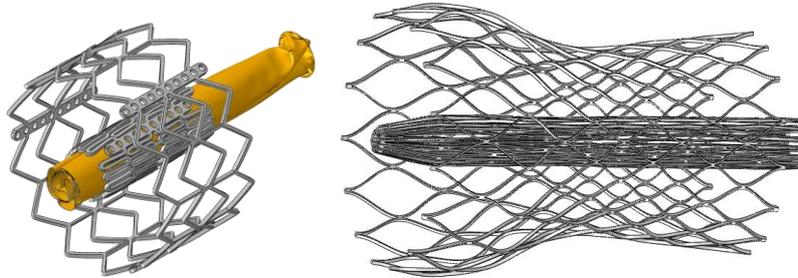
**Fig. 1 Edwards *Sapien* (left) and Medtronic *CoreValve* (right) in their initial and crimped positions. The deflated balloon is also shown on the left with cross-section to demonstrate the folding.**
