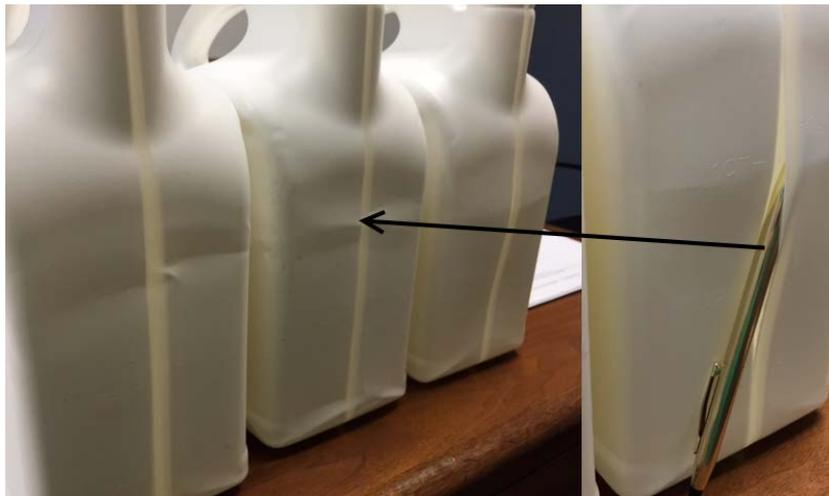
Figure 1: Rupture area on a drop tested 1 gallon container
