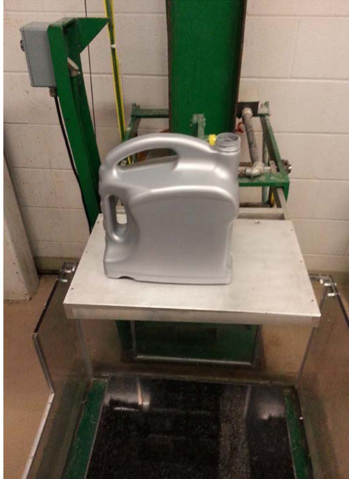
Figure 2: Drop test apparatus
