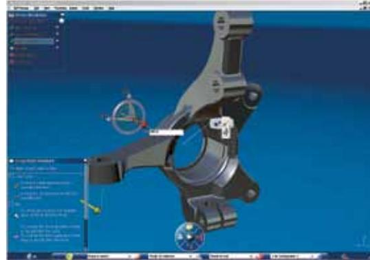
*Using DesignSight Structure, the designer interacts with the robot to define the load application location, orientation, and magnitude on the steering knuckle.*
