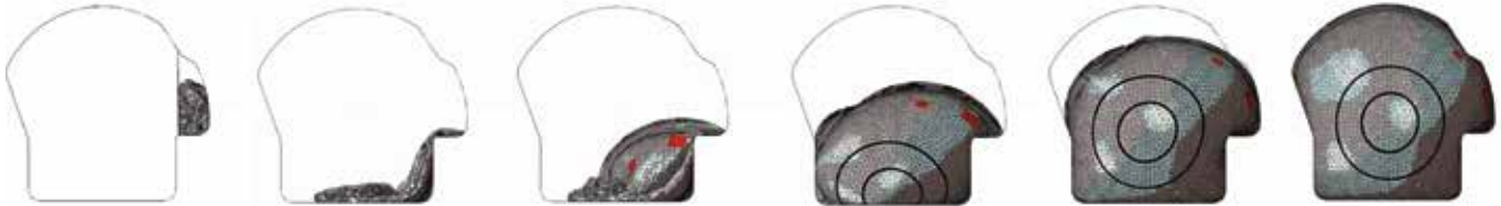
Figure 3. The simulated deployment of the inflatable plug closely matches the deployment of a plug in a full-scale test.
