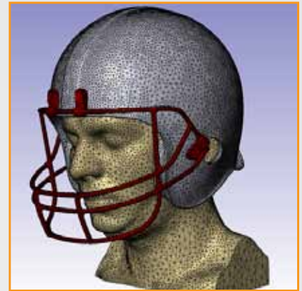
FE mesh of NRL-Simpleware head model with football helmet
