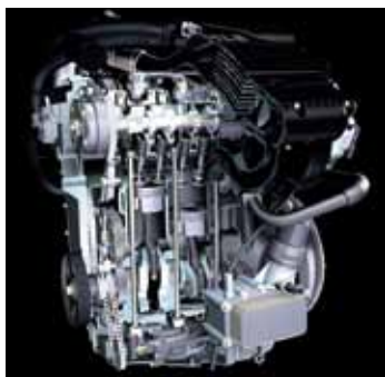
Figure 1. The 3-cylinder design for MAHLE's downsized engine (shown here in cross section on left) generates the power of a 6-cylinder engine, necessitating the need for structural and thermal optimization (right) to ensure that the engine can sustain the stresses of running at higher loads.
