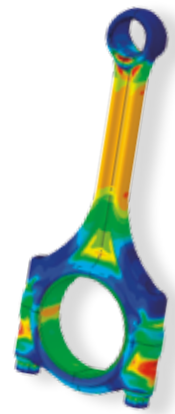
Figure 2. Abaqus FEA was employed extensively for structural and thermal analyses during the design of MAHLE's range extender (REx) engine for electric vehicles. Pictured is the engine assembly finite element model and temperature distribution (left), stresses on the engine block and crankcase (center) and connecting rod stresses due to combustion pressure (right).
