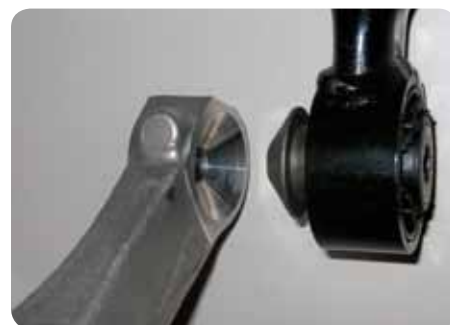
Figure 1. Close-up view, before assembly, of the toe-link (black) and the rear knuckle (silver) using a conical joint.
