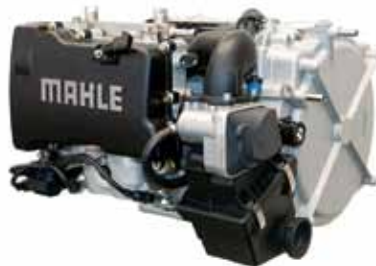
Figure 3. MAHLE's REx is a gasoline-powered engine that is used to recharge the batteries of a more traditional electric-powered vehicle. To arrive at a durable, lightweight carry-on-luggage-size footprint, designers used extensive structural and thermal simulation in conjunction with optimization studies.
