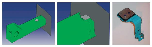
Crushing of a composite cone structure with a rigid insert bonded into a cutout in the cone is simulated in CZone for Abaqus. As the impactor reaches the bonded insert, a fragment including the insert and portion of the cone breaks away from the structure, comparing well against a similar fragment that is produced in the experimental test.
