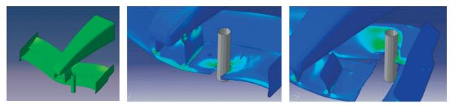
The composite front wing for an F1 race car is impacted against a rigid pole. Progressive crushing of the wing occurs as the pole penetrates through the wing. Significant forces are also transferred through the structure, causing the wing to then break away from the vehicle.
