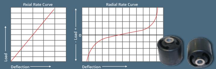
The bushings that attach the lower control arm to the frame are modeled using a linear stiffness in the axial direction and a nonlinear stiffness in the radial direction to simulate the bushings' carefully-tuned behavior.
