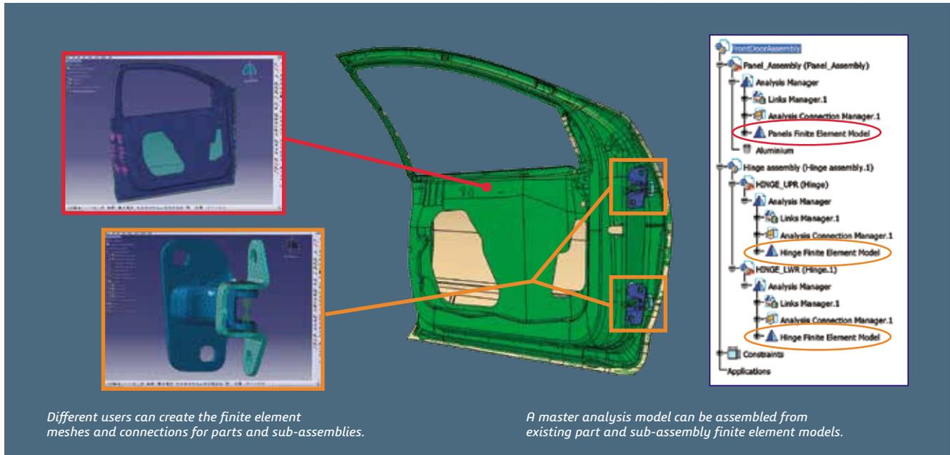
*Different users can create the finite element meshes and connections for parts and sub-assemblies.*
