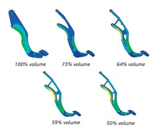
This nonlinear brake pedal example shows the progression of a topology optimization as it attempts to maximize the stiffness while reducing the volume by 50% during 31 design cycles.
