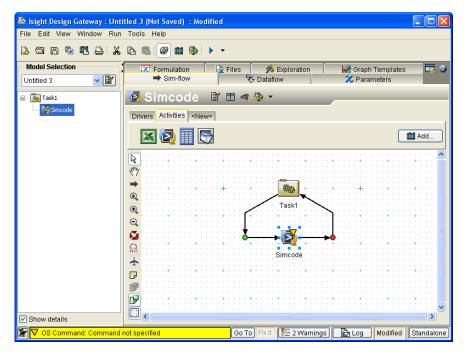
The Simcode component executes an external program from within an Isight model. The program's input is one or more files. Parameter values are written to the files to allow the model to vary the inputs. Similarly, the program's output consists of one or more files. Values are read from these files and stored in parameters so they can be used in other parts of the model.
