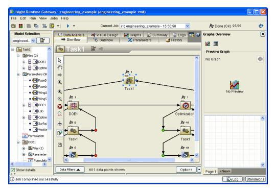
The Runtime Gateway provides access to graphs and tables that allow you to view execution information. You can also view data using the tabs on the Runtime Gateway itself.
