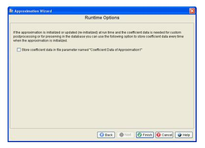
The **Store coefficient data in file parameter named** option creates a file parameter that stores the approximation's coefficient data. This option is useful if the approximation is initialized or updated (re-initialized) during execution and the coefficient data is needed for custom postprocessing. It is also useful if you want the coefficient data preserved in your database.
