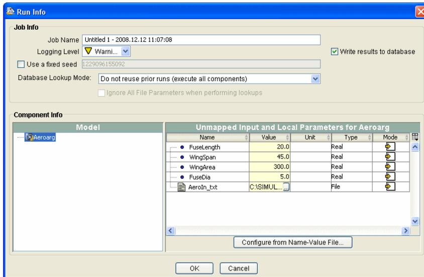
This interface allows you to enter values of interest for the input parameters prior to running the simulation code.
