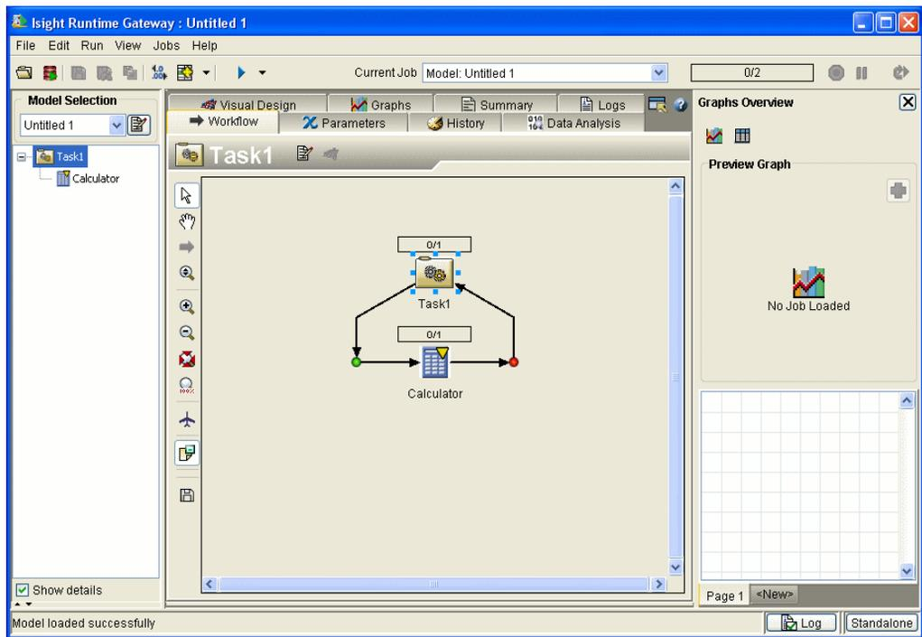
This interface differs from the Design Gateway in that it allows you to control execution and view results, but it only allows limited access to components and the workflow. It also lets you create graphs and tables, view parameter information, create approximations, access data analysis tools, and resubmit models for execution. The following main features are available:
