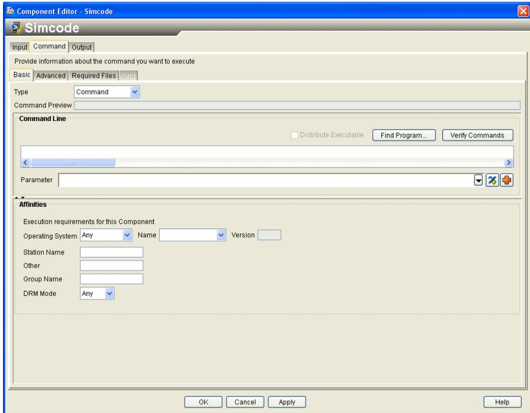
By default, the Command tab is selected. There are four different subtabs available from the Command tab: Basic, Advanced, Required Files, and Grid (if available). The Basic tab is selected by default. The Command Line text box is used to enter the program name, path of the program, name of the input file, and the name of the output file.
