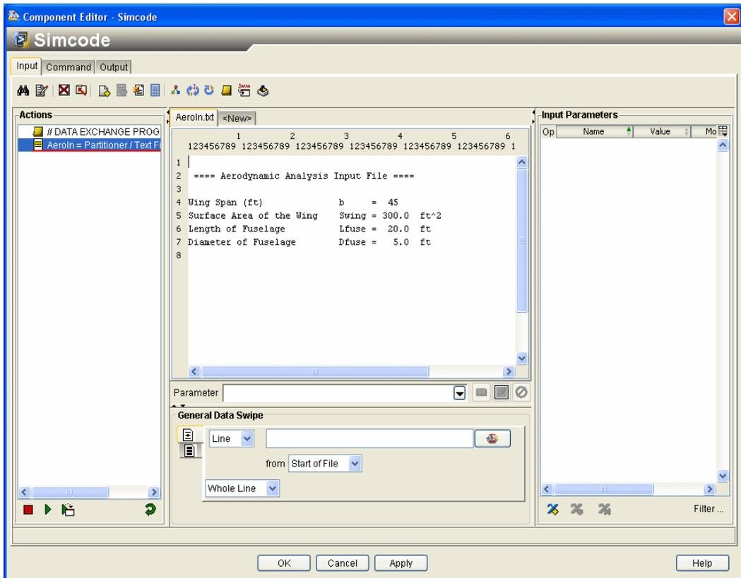
The left side of the editor shows the current list of actions for the file. The center of the editor shows the contents of the template input file used by the simulation code. The right side displays the input parameters with properties such as Mode, Type, etc. Since no parameters have been defined yet, this area is blank.
