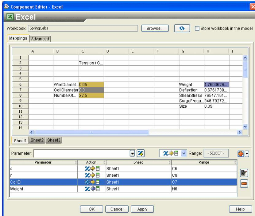
Instead of typing the names of all the parameters that you want to specify, you can use the name-value mapping option and make use of the fact that some of the cells contain text describing the values in the adjacent cells. You will now use name-value mapping to map the remaining parameters in the workbook.
