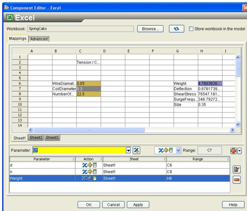
2. Type `CoilD` in the yellow **Parameter** text box. This action assigns a name to the parameter.
