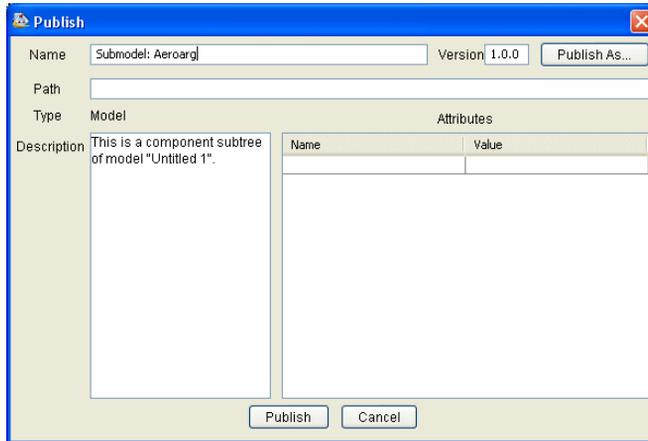
The component, by default, is named *Aeroarg*. You can change the name and change the description, if necessary, in the corresponding text boxes.
