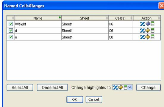
This dialog box shows how Isight will automatically create parameters based on the named cells in Excel. Three of the cells are named *Weight*, *d*, and *n*. The cells that have these names are described in the window. By default, Isight will create parameters *d* (WireDiameter) and *n* (Numberof) as input parameters (as shown in the Action column), and the parameter *Weight* as an output parameter.
