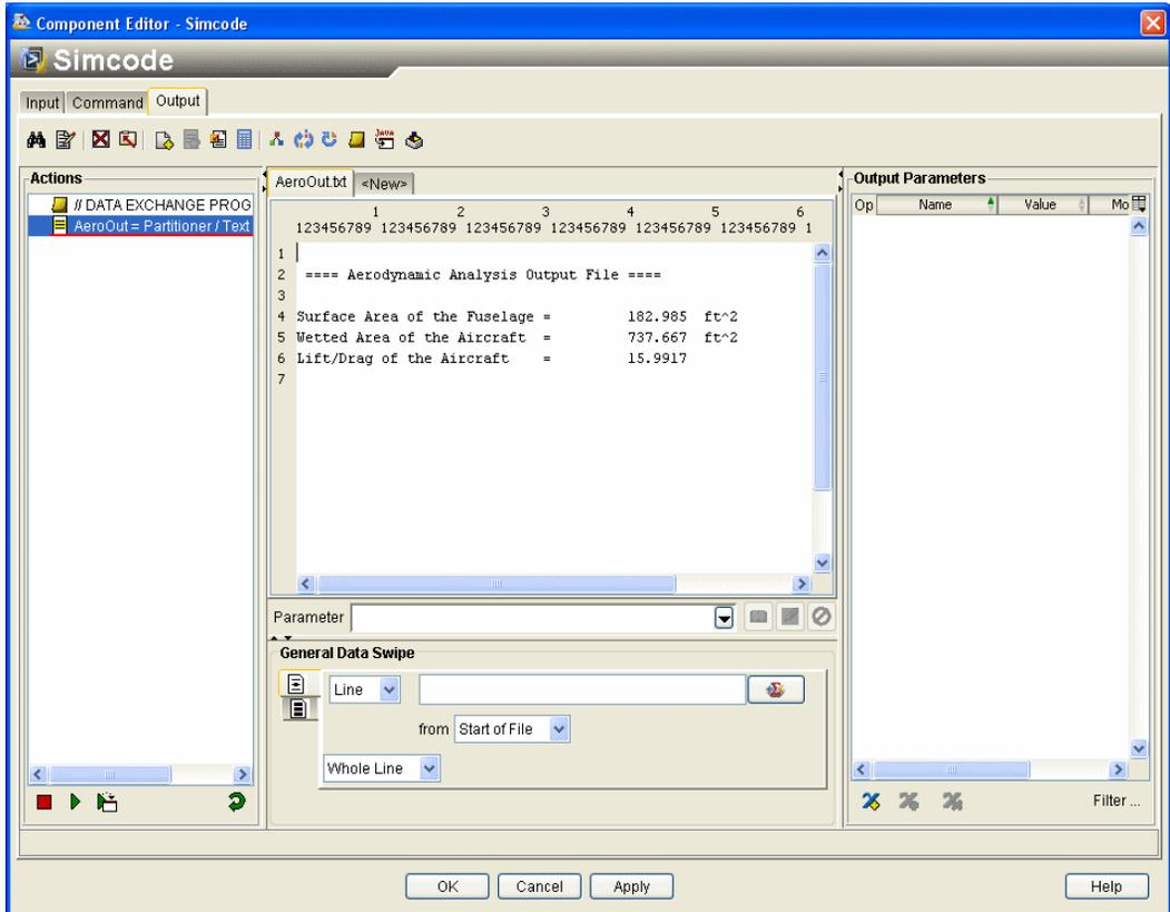
The left side of the editor shows the current list of actions for the file. The center of the editor shows a copy of the output template file. The right side displays the output parameters. Now you need to specify the output parameters using the same procedure as used to specify the input parameters.
