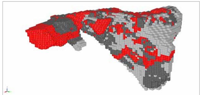
Resource block model, created in Surpac 6.7, which is colored by material class: waste, low grade, high grade.
