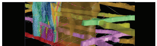
Surpac at a base metal operation. View drillholes, under-ground workings, ore zone and resource block model.
