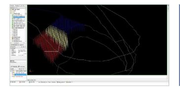
Surface mining - efficient design of bench blast patterns considering blast hole layout, load and charging, detonation sequence and blast solids
