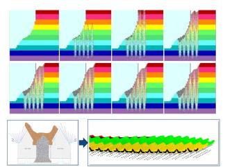
Create realistic undercut sequences in PCBC with operational constraints
