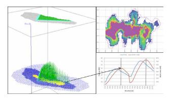
Find the best elevation and orientation for locating a new extraction horizon for block and sub level caves
