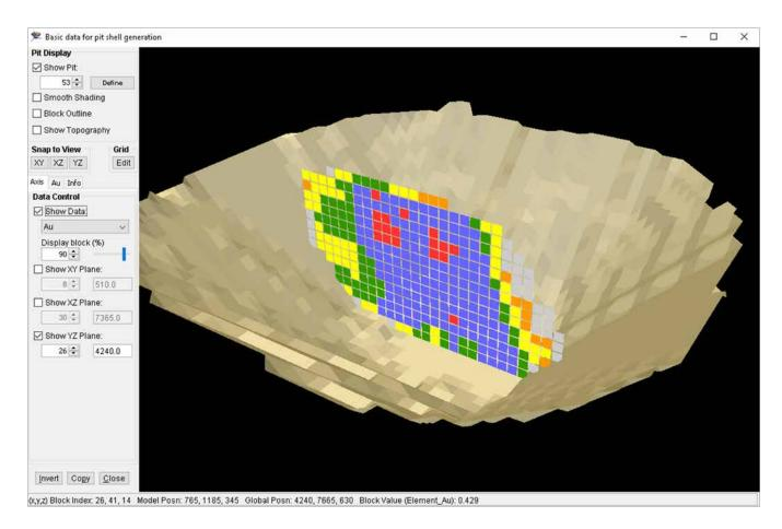
The Pit Optimizer is the foundation of GEOVIA Whittle™. Designed to produce a seamless workflow, the Pit Optimizer provides tools for importing data, manipulating resource models, modelling pit slopes, performing pit optimization, and analyzing results.
