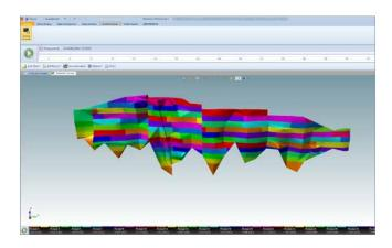
This will provide greater flexibility to Mine Planners when exploring a range of mining methods for their optimized Stope shapes.
