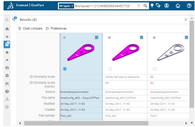
Side-by-Side Part Comparison based on attributes and shape similarity, with color coded differences and multiple criteria sorting
