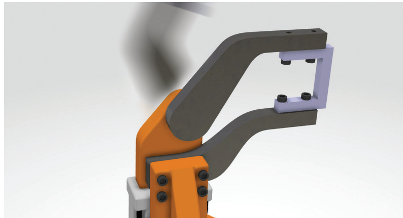
DELMIA Device Task Definition delivers the capability to program and simulate forward kinematic mechanical devices.
