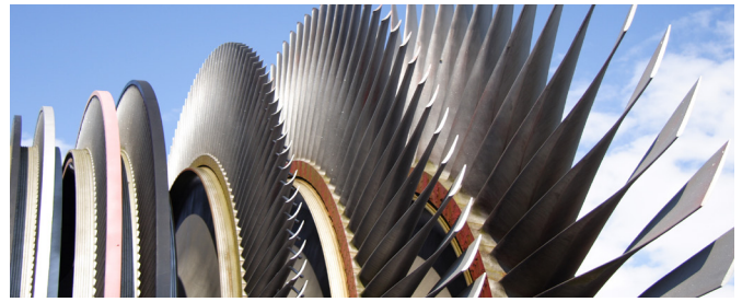
Blades from a typical thermal power plant steam turbine
