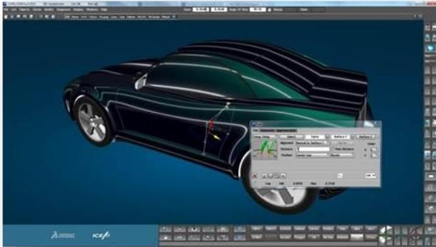
An add-on module to ICEM Surf Professional, ICEM Surf Master extends the capabilities for global modification, creation and diagnosis of surface geometry focusing on global filleting, overcrowning and global connections of surfaces, enabling existing designs to be quickly and easily modified for consistent design integrity and engineering data re-use.
