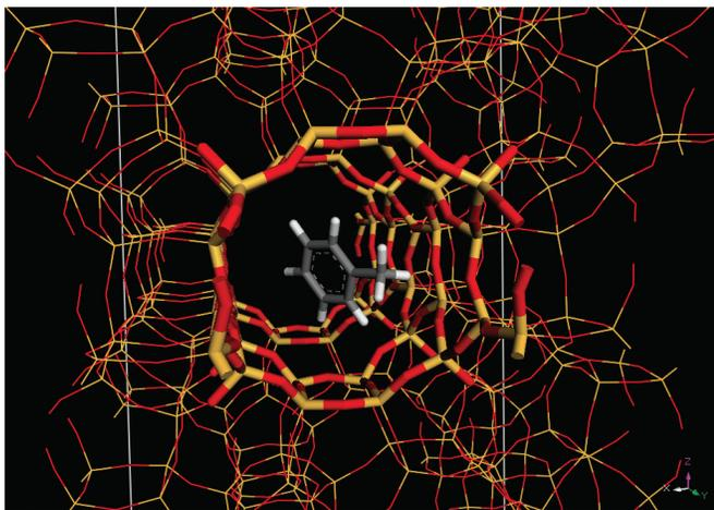
**Figure 1:** BIOVIA Materials Studio Adsorption Locator can be used to find the most stable adsorption sites for a broad range of materials. The image shown here illustrates the most stable configuration of toluene adsorbed in a BEA zeolite pore.
