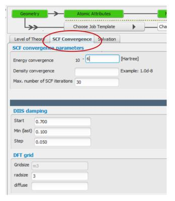
Energy and/or density convergence criteria can be entered in this panel. A density convergence criteria is useful for properties and methods that need a very accurate density like post-Hatree-Fock methods or TDDFT.
