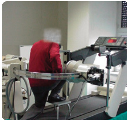
Post-surgery patient undergoing videofluoroscopic analysis of the function of their replacement knee. Image courtesy of Dr. Sergio Romagnoli.
