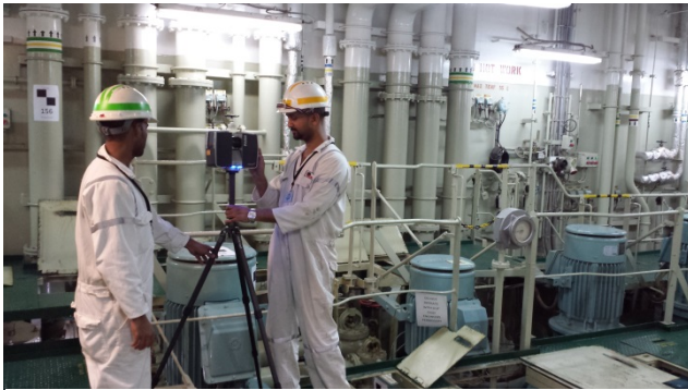
ASRY is using 3D scanning technology to carry out engineering assessments for installing ballast water treatment systems on ships (photo: ASRY)
